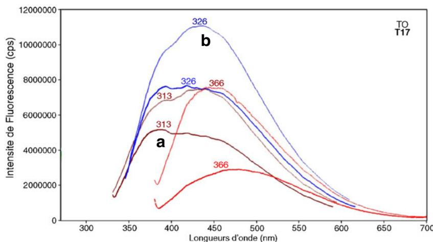
Linseed oil deposited on glass slides 1 year before and then kept under daylight at room temperature ( $T_0$ ) has been submitted to three series of irradiation (Tables 1 and 2). The layers of oil were not really regular, neither still dry.
